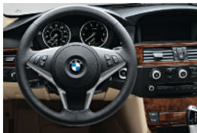
3-spoke leather-wrapped multi-function sport steering wheel lets you keep both hands on the wheel while adjusting various comfort functions, such as radio stations, CD selections and volume.
