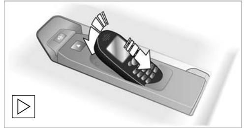
2. Insert the mobile phone and press down lightly until it snaps into place.
