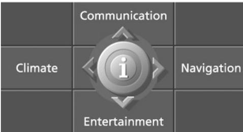
2. Move the controller forwards to open "Communication".
