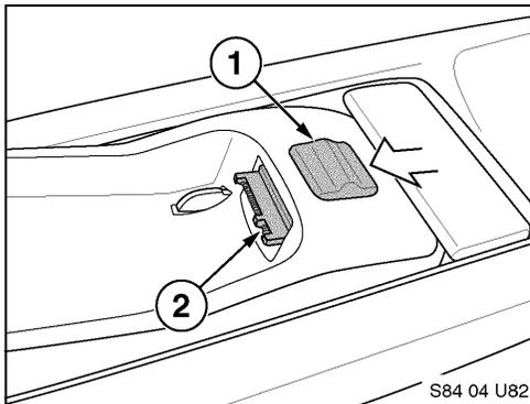
When using the **V60S** move button (1) to the back position. This will raise the connector (2) to the correct position in order to insert the handset.
