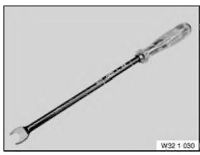
Note: For disconnecting hydraulic lines from steering
