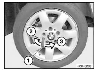
Turn adjusting screw with a screwdriver until the wheel is no longer able to turn.
