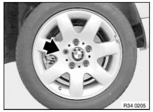
Completely unscrew one wheel stud on each rear wheel.
