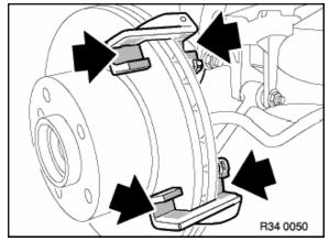
Clean brake caliper mounting bracket at hammer head guides and apply a thin coating of anti-squeak compound.
