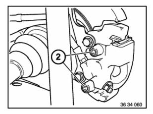
Release guide screws (2) with special tool 34 1 080 .
