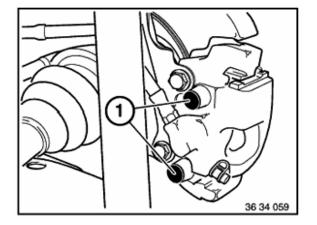
Remove plastic plugs (1). Right side: Disconnect plug connection for brake lining wear sensor.
