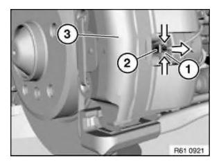
Press clip (1) together and detach brake pad sensor (2) in direction of arrow from brake pad (3).
