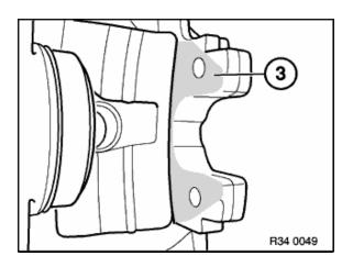
Clean contact face (3) of brake caliper and apply a thin coating of antisqueak compound.
