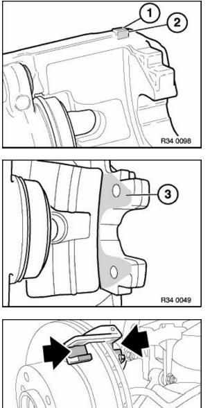
Clean mounting faces (1) and (2) of brake lining hammer heads/brake caliper housing and coat with anti-squeak compound.
