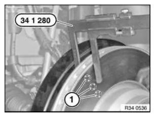
Remove outer brake lining.
