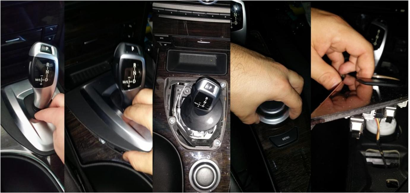
14.) Route the wire towards the shifter. Now remove the plug in the red circle and connect the T-Harness from the kit and also connect the wire from step 13 to the harness.
