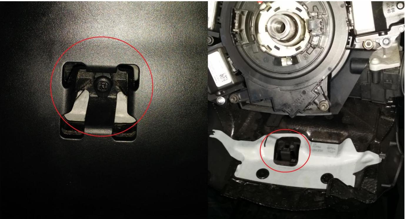
11. Gain access to the rear of the steering assembly and locate the black plug. Remove the plug and open the tab on the plug. Then insert the loose wire leads included in the kit into the plug as shown into position 12 and 13.
