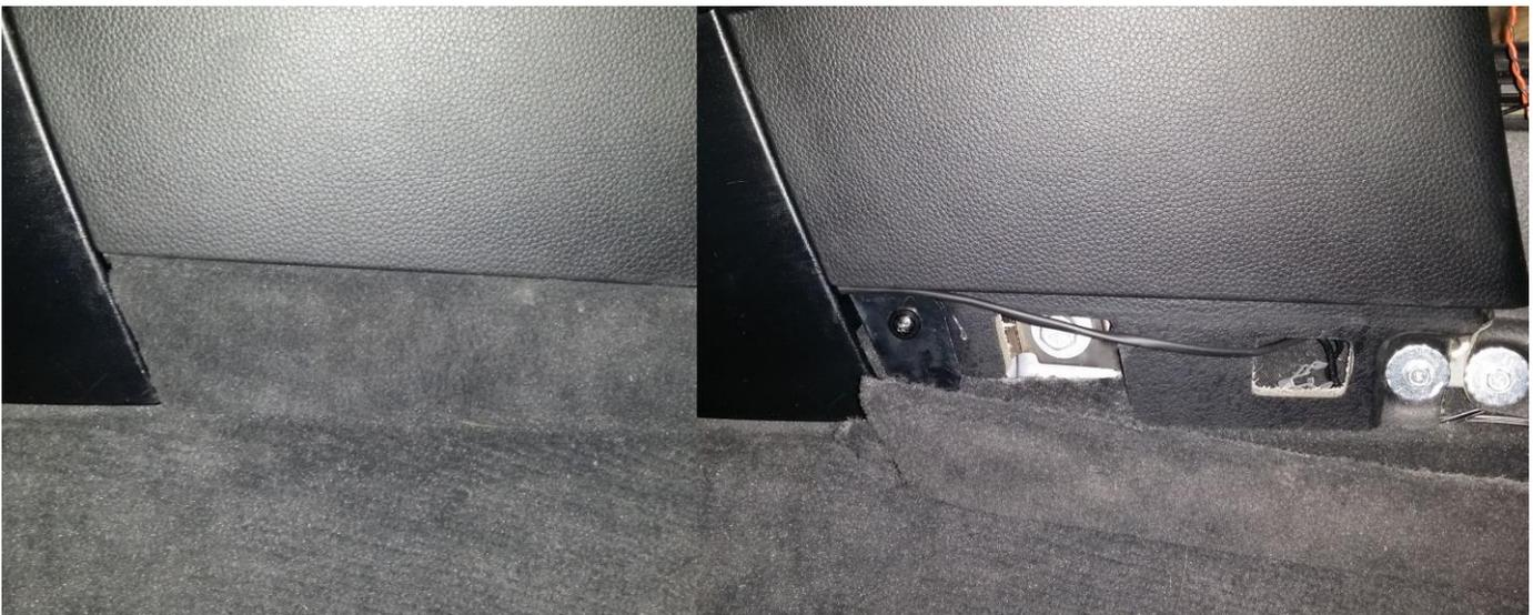
13.) Reach into the inner lip of the shifter and pull up releasing and removing the baseplate. Remove the Idrive controller by pulling straight up. Remove the center armrest area by pulling up and disconnecting the wiring underneath.
