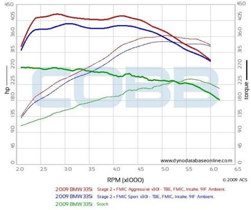
Above are the dyno results for a 2009 BMW 335i MT on our in-house Mustang AWD Dynamometer. Results may vary based on conditions such as particular model of vehicle, fuel quality, etc.
