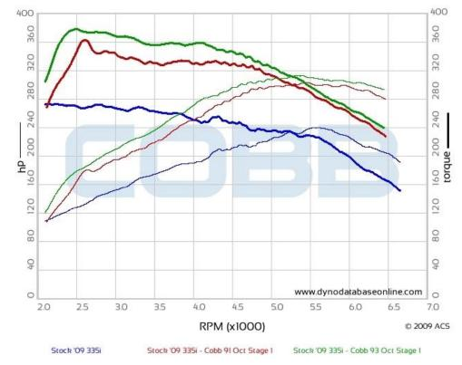
Above are the dyno results for a stock 2009 BMW 335i MT on our in-house Mustang AWD Dynamometer. Results may vary based on conditions such as particular model of vehicle, fuel quality, etc.
