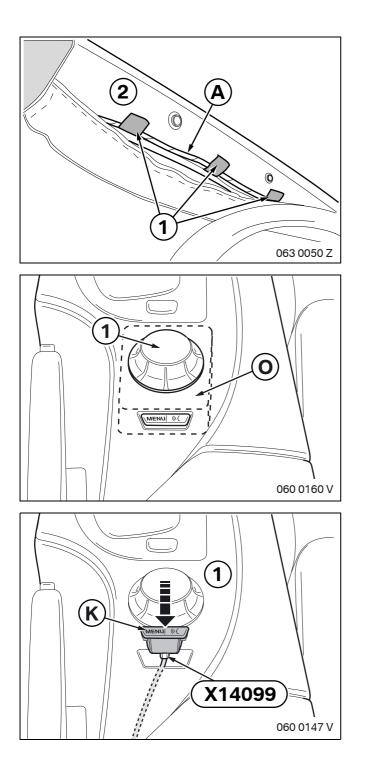
Secure wiring harness **A** to the left A pillar (2) using textile adhesive tape.
