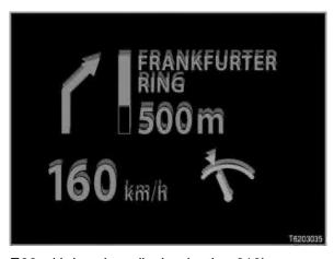
f a conventional windscreen is used, the projected image will be reflected onto both the inner and outer glass. This overlap will cause a double image.
