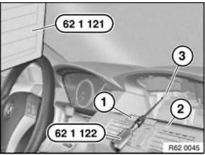
Check height adjustment using scale on special tool 62 1 121 . If height adjustment is not correct:
