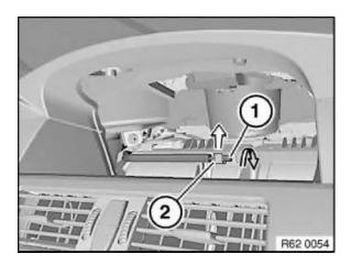
Unclip flexible shaft (1) in direction of arrow from holder (2).
