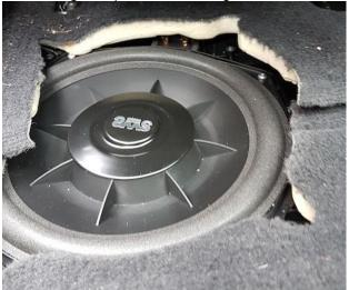
As stated in the fitting guide a grille spacer must be used so that the subwoofer voice coil does not hit the OEM grille when refitted and being driven 'hard'. Not readily available off the shelf I decided to order two 10mm thick 'A4' sized sheets of Perspex from Trent Plastics. The 'A4' sheets arrived the next day...
