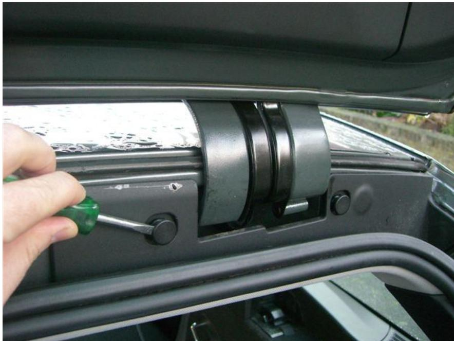
Now the cover is removed. Next step is to remove the plastic plug that holds the lower part of the rightmost wire guide:
