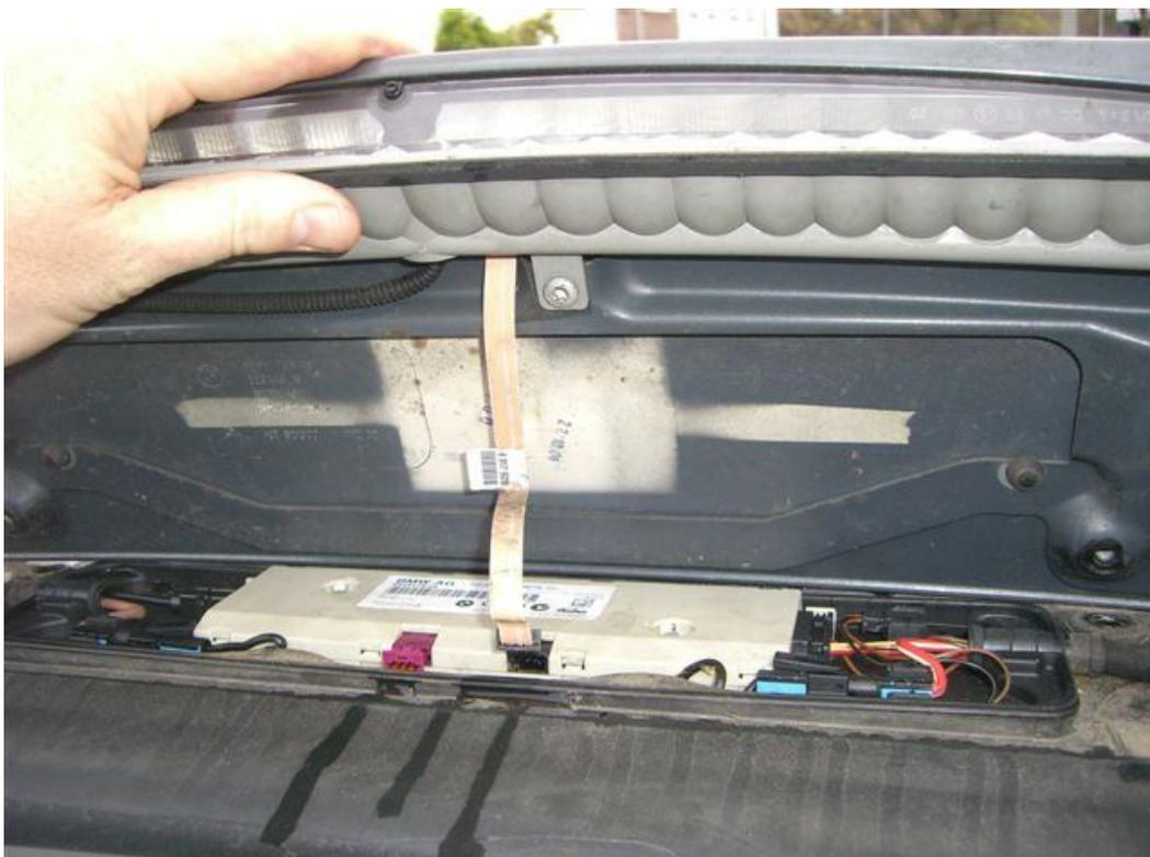
I removed this antenna cable, and on the right hand side I unplugged the high breaking light connector:
