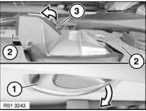
Unhook Bowden cable for release lever:
