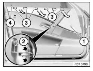
Carefully unclip door trim panel (1) at top from retainers (3). Feed door trim panel (1) upwards out of central clip mounting and release button (4).
