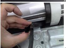
use a very thin flat head screw driver to separate the holder at the clip on points. Be very carefull about your own fingers while doing this. You may need another bigger screw driver to assist. It is made of two part channels.
