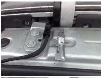
undo the small nut to release the cable holder.
