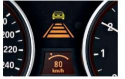
□ Active cruise control with Stop & Go function enables comfortable driving at a preset speed (30–180 km/h). When driving in columns of traffic, your BMW automatically adapts to the speed of the preceding vehicle and maintains a preset distance.
