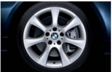
□ BMW light-alloy wheels star-spoke 124 with runflat properties and mixed tyres, 8 J x 18 inch, 245/40 R 18 tyres at the front, 9 J x 18", 275/35 R 18 tyres at the rear (with wheel locking bolts).
