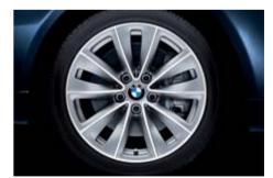
□ BMW light-alloy wheels double-spoke 247, forged, with runflat properties, 8 J x 18 inch, 245/40 R 18 tyres (incl. wheel locking bolts, slate grey rims, part-polished).
