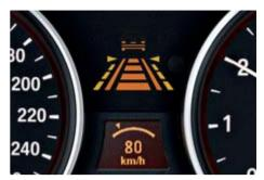
□ Lane-keeping support uses a camera to monitor when the vehicle is approaching lane markings, and immediately warns the driver via a steering wheel vibration. The system is designed for cross-country highways and motorways, and is switched on and off with a button in the multifunction steering wheel.
