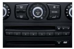
■ Functional bookmarks: The driver's and passenger's most frequently used navigational targets and telephone numbers or specific CD tracks can be individually stored on eight separate buttons and accessed with one click.
