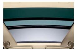
□ Panorama glass roof with generous opening and viewing area as well as speed-dependent wind deflector. Both glass sections can be raised via electric fingertip controls, the front part has an additional sliding function, electrical sun shade as well as comfort opening/ closing function with trap release.
