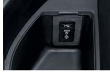
□ USB/audio interface in storage compartment under the central front armrest for USB connectivity and playback of e.g. MP3 audio files.
