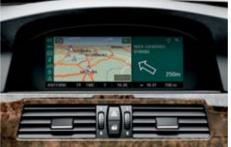
□ Navigation system Professional\* with 8.8" colour display, navigation based on voice output and arrows or route map. Using the splitscreen function, different functions such as radio and navigation can be displayed side by side. □ Navigation system Professional\* with integrated Bluetooth mobile phone preparation for telematics services.
