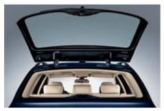
■ Rear window, can be raised separately: opens separately for quick and easy access to stored objects.
