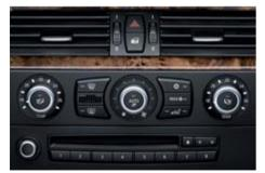
□ Automatic air conditioning, extended with AAR, solar sensor and fogging sensor, automatic temperature control and air distribution (separate for driver and passenger), also air volume control; status and settings shown on the Control Display. With adjustable armrest and air-conditioned storage tray in centre console (standard on 550i and 535d).
