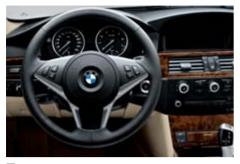
□ Leather sports steering wheel, very comfortable grip thanks to small diameter (379 mm), three spokes, with multifunction buttons; the integrated buttons can be used to operate the radio, CD drive and telephone (optional) while on the move. Two buttons are available for userdefined functions.
