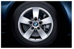
■ BMW light-alloy wheels star-spoke 242, 7 J x 16 inch, 225/55 R 16 tyres (incl. wheel locking bolts (standard on 523i, 525i, 520d and 525d).
