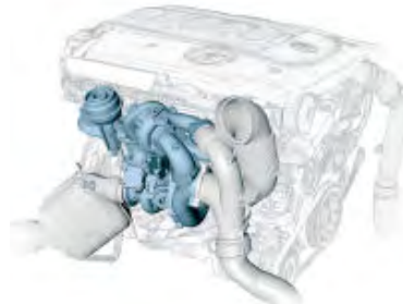
Fast buildup of pressure: the two parallel turbochargers (shown in blue) make a key contribution to the outstanding responsiveness of the 535i xDrive's inline six-cylinder engine.
