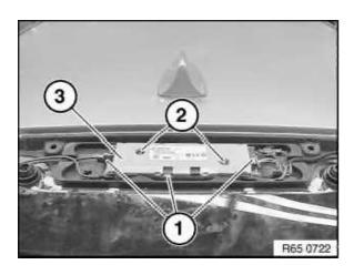
Unlock plug connections (1) and disconnect. Release screws (2). Lift out antenna amplifier (3).
