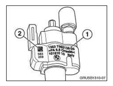
2. Check each injector's part number and index number (indicated as # 1), which are located on the injectors' plastic housing facing the ignition coil.
