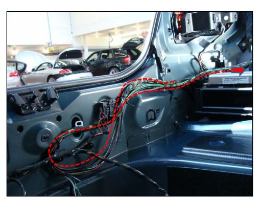
5) Route the harness for the MULF in a loop on the tail panel, as shown. This way, the harness will not have excess slack in it, and will allow the MULF to sit on top of the bracket in the left side of the luggage compartment.
