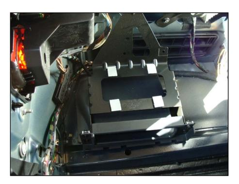
4) Secure the hook side of 2 pieces of Velcro to each other. Repeat 3 more times (using 8 pieces of Velcro in total). Peel the backing off one side of each Velcro pair and secure each to the bracket in the left side of the luggage compartment, as shown.
