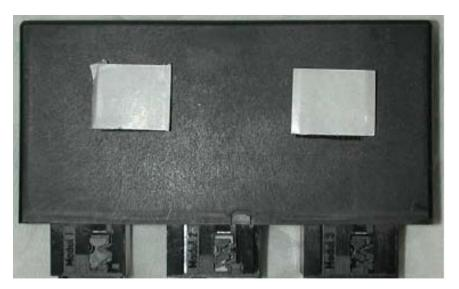
2) Secure the hook side of 2 pieces of Velcro to each other. Repeat once (using 4 pieces of Velcro in total. Peel the backing off one side of each Velcro pair and secure each to the back side of the PDC module, as shown.
