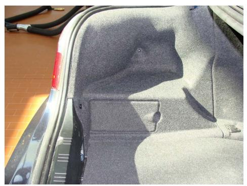
8) When reinstalling the luggage compartment trim panels, install a new left side panel, which has a shelf as opposed to an oddments tray.
