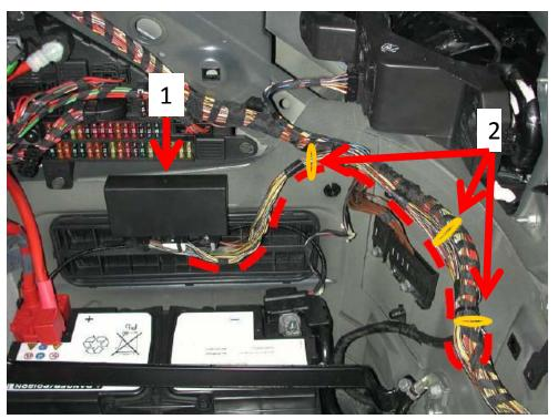
3) Route the PDC module (1) back along its own wiring harness to reach the point above the middle of the right side air extractor. Peel the backing off of the Velcro pads and secure the PDC module to the body structure. Secure the wiring harness with 3 wire ties (2). Replace any panels that have been removed.
