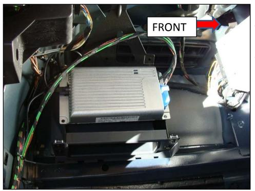
7) Remove the adhesive backing from the 4 Velcro pads and place the MULF on them, oriented with the connectors toward the front of the vehicle.
