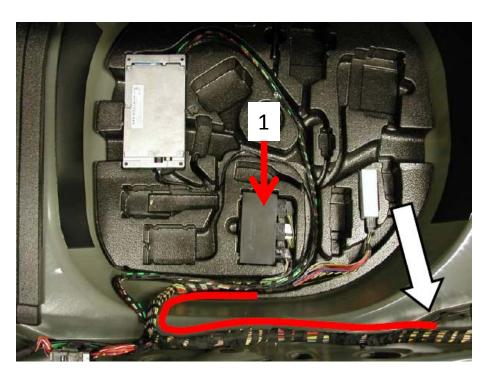
1) Remove the PDC Module (1) and pull the wiring harness back along the red line to the point identified by the arrow.
