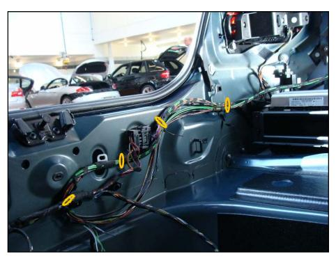
6) Secure the harness in its new position, using 4 wire ties.
