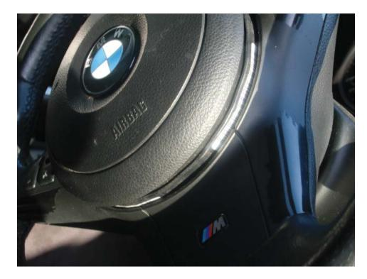
Once the airbag is released pull it forward & move it to one side but **DO NOT UNPLUG THE WIRES CONNECTED TO THE AIRBAG**
