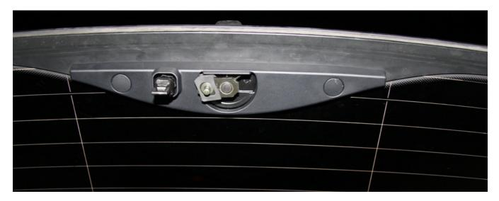
Use a fine screwdriver or knife to pry out the two black round covers so you can access the nuts below.
