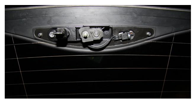
Now you slide off the black electric connector and gently pull the axle assembly out of the hole in the glass. Throw away the defective micro switch, replace with the new micro switch. Reconnect the plug and put the axle assembly back in the hole. I forgot to take pictures of this but it is straightforward once you get to this step as all is loose and requires not tools or special knowledge to deal with.
