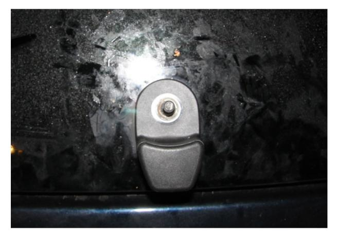
You can now simply pull the micro switch off the axle and in doing so, you will notice a wire which goes through the hole in the glass, so you will now need to open the glass to access the box on the inside of the glass.
