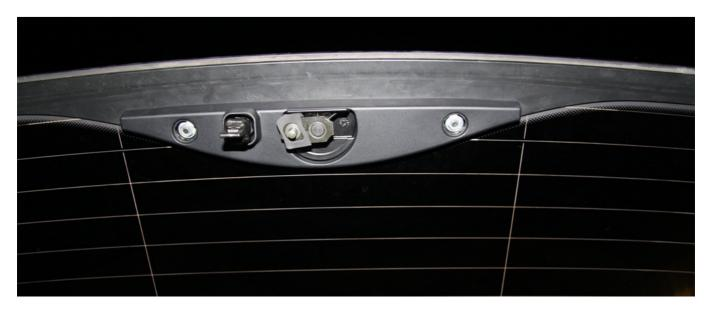
Now use the 10mm socket wrench to remove the two nuts and then gently take off the plastic cover.
