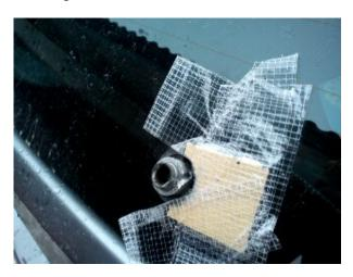
5. Be sure that the cut made by Dremel is all the way down and now use a flat screw driver to "open" the metal washer to take it off the axis.
