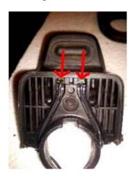
Micro switch housing is very sensitive for water. This type of switch is normally used in cheap indoor applications like a keyboard for a table calculator or a remote control. Poor quality as usual=BMW.
