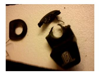
4. No comes the most tricky part. The metal washer is still on the axis...protect the glass and make a cut with the Dremel-tool. In my case I used tape and a piece of wood to protect the glass.
