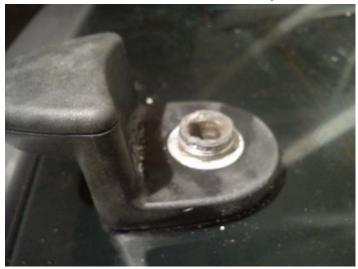
3. Protect the glass and use the dremel-tool. Make a cut on both sides and bend/pull of the plastic part of the micro switch. Cut the cables. Don't cut in the glass...it will crack=expensive!
