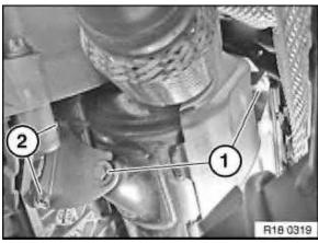
Release catalytic converter suspension bolts (1).
