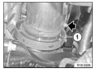
Release screw on turbocharger flange.
