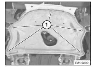
Release screws (1) and remove reinforcement plate.
