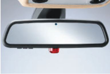
Automatic-dimming rear-view mirror senses the bright headlights of vehicles behind you, and automatically darkens.
