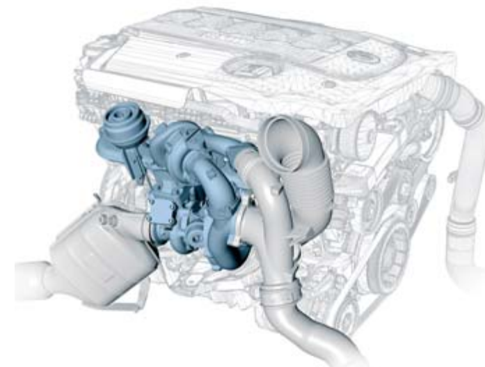
Fast buildup of pressure: the two parallel turbochargers (shown in blue) make a key contribution to the outstanding responsiveness of the 535xi's inline six-cylinder engine.
