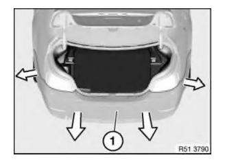
Unclip bumper trim (1) to side panel (1) on left/right outwards. Remove bumper trim (1) in direction of arrow towards rear. <u>With optional extra PDC:</u>
