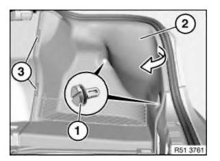
Open rotary clips (1) and remove.
