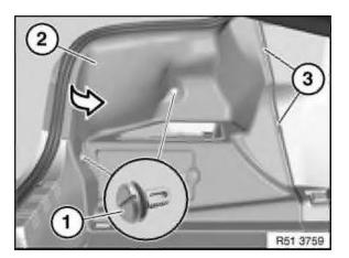
Open rotary clips (1) and remove.
