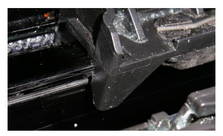
Step 5: Take a Dremel tool (or look-a-like) and <u>cut away</u> the triangle shaped front corner of the drive cable plate.
