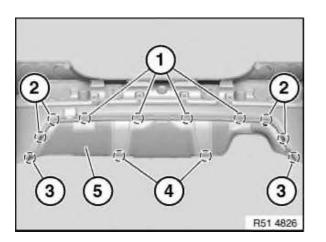
Release retaining elements (1, 3 and 4). Release catches (2) and remove diffuser (5).
