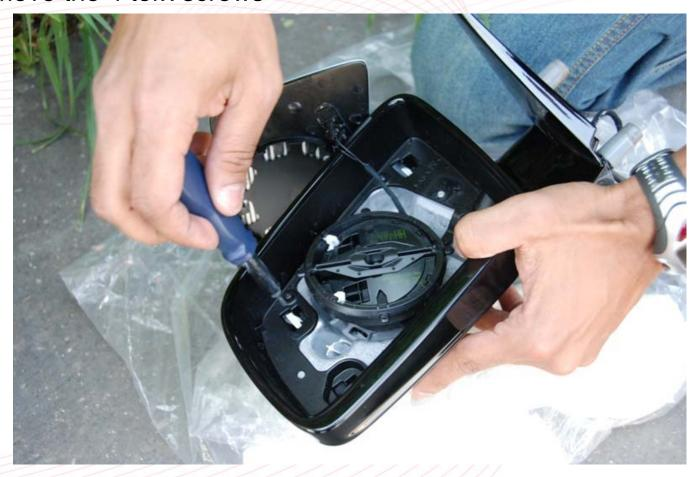
Unscrew motor of the mirror – torx screw.
