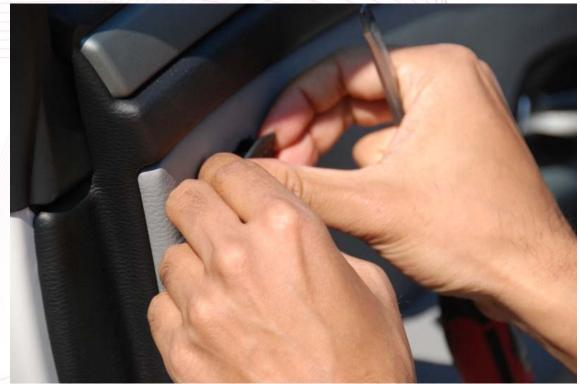
Remove light cover at the bottom. Just use screw driver
