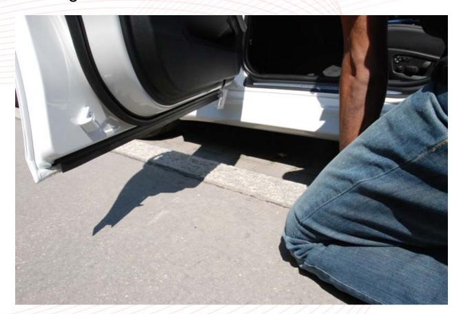
Remove cover of a TORX screw near the hinge of the door.
