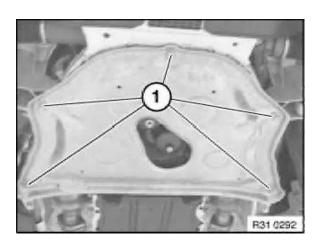
Release screws (1). Remove reinforcement plate. *Installation:* Tightening torque 31 10 9AZ .
