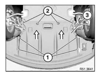
Release screws (1) and (2) and pull out underbody protection (3) from under bumper trim.
