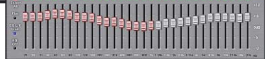
EQ of the filtered Low Pass Front Woofer. Select All on, equalization performed moving the cursors all together
