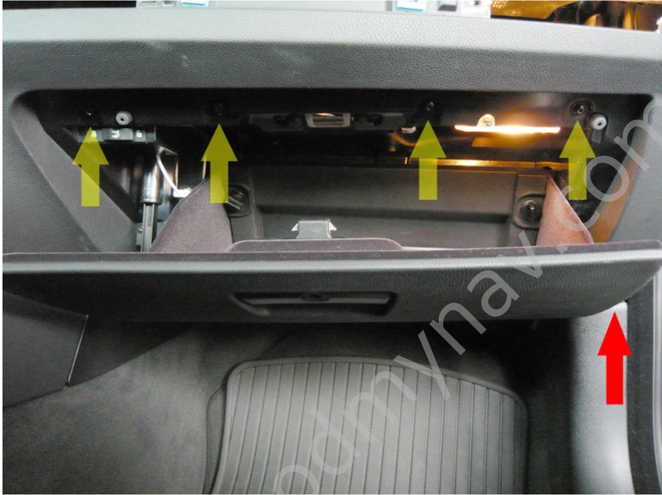
8. Open the glove box and remove 7 screws
