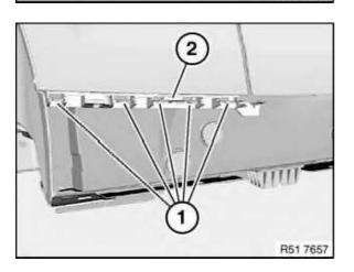
Installation: Catches (1) on holder (2) must not be damaged.
