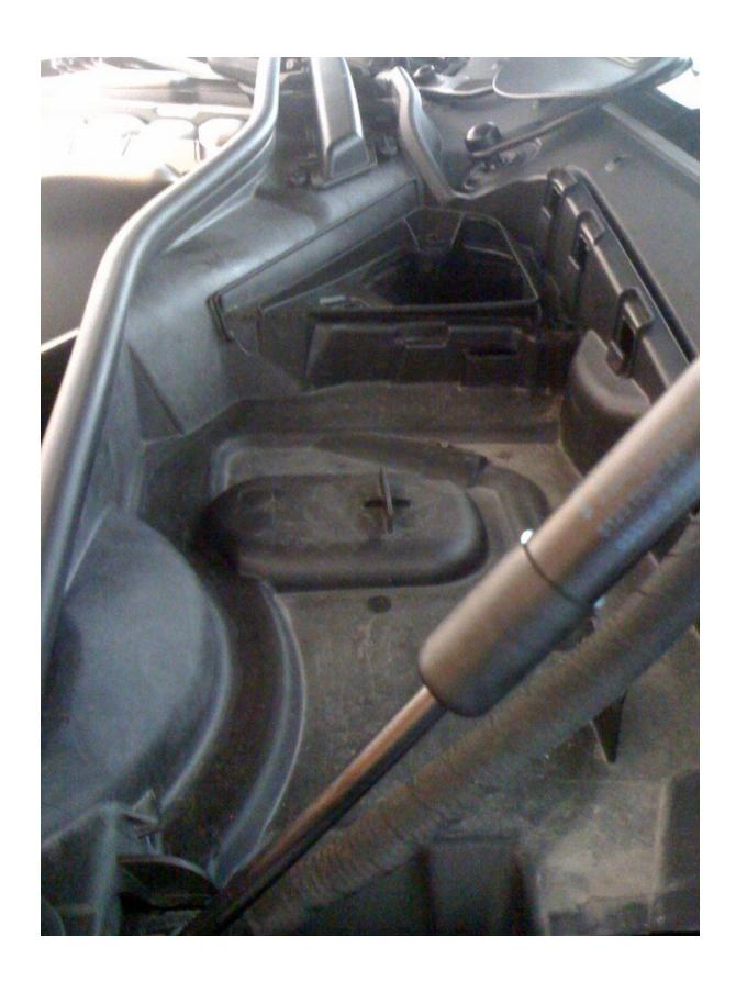
Step 6: Release one last 13mm lock right near the joining area of the cowel area. The pull the cowel section out by pull it up and toward the passenger side of the car. Step 7: Release the sensor connector (Not in picture) that plugs onto the lid of the fluid reservoir.
