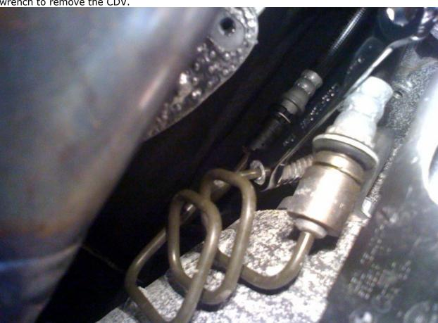
Step 13: Replace the CDV with the modified unit and then reconnect the hardline.
