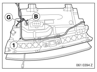
Use cable tie  ${\bf G}$  to secure connection cable  ${\bf B}$  to the standard wiring harness (1) to act as strain relief.
