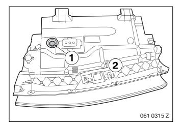
Drill through the glove compartment (2) in the middle of the marked area (1) using an 18 mm step drill bit.
