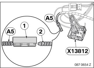
Unlock the fiber optic cable connector (1) on branch **A5** and connect the disconnected fiber optic cable (2).
