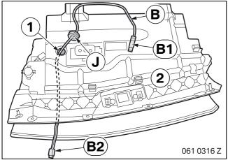
Install connection cable **B** as follows:
