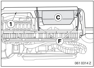
Secure interface **C** to the support (1) using cable ties **F**.
