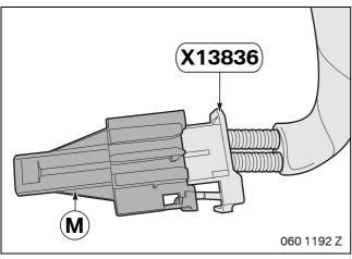
Replace flash adapter casing on fibre optic cable casing X13836 with short circuit casing M.
