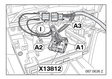
Disconnect the following cables from plug **X13812** (black 16-pin) of the ASK or CCC and connect to socket casing **I**:
