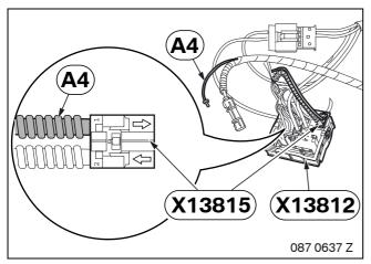
Unclip fiber optic cable casing **X13815** (black 2-pin) from plug **X13812** (black 16-pin) of the ASK or CCC.
