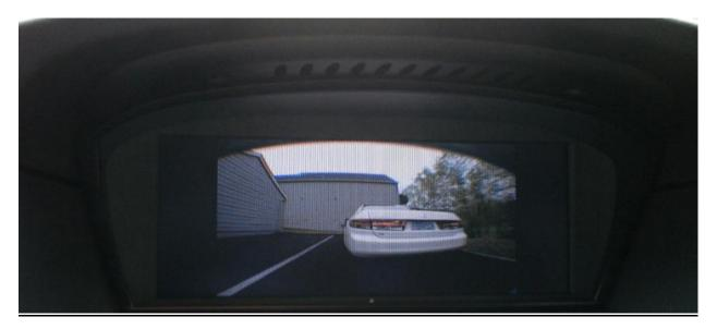
Side View Camera shows cars to the left and right and shows how close you are parked to the curb, Side View camera option is on by default in the ACM but has to be operated by a switch since this is after market Eclipse camera, excellent picture quality for this camera also
