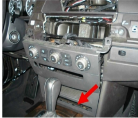
Pull out the Control Board carefully.
