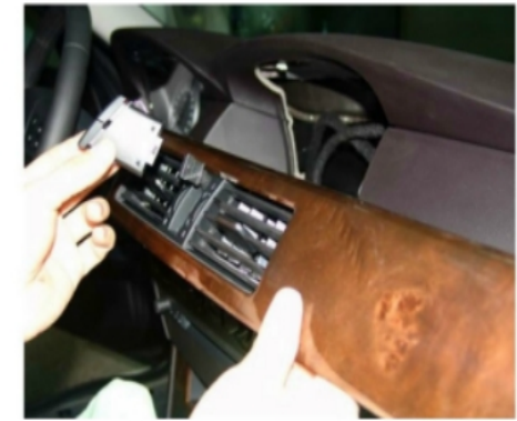
Remove the cover after unplugging the connector.
