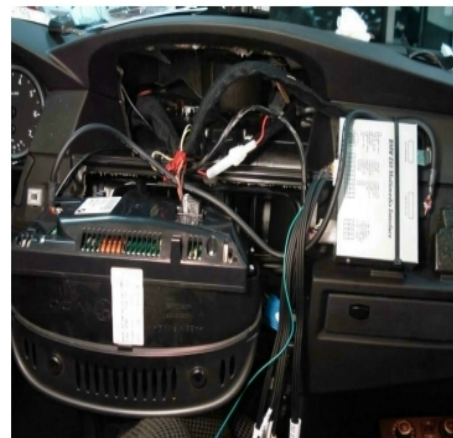
Fix all the wirings, put the monitor and the control board back to complete the installation process.
