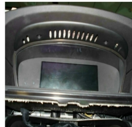
Fix all the wirings, put the monitor and the control board back to complete the installation process.
