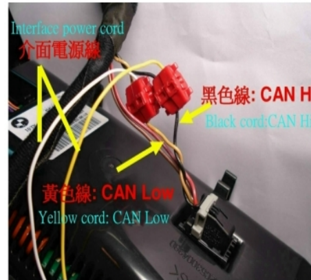
Black and Yellow cord of the monitor's power cord should be connected to the Yellow and White cord of the Interface's power cord correspondingly.
