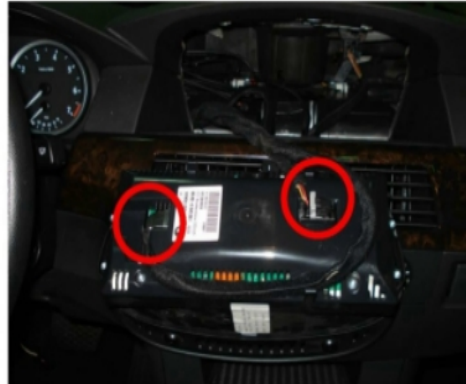
Loosen the screws of the monitor as indicated, remove the monitor, and unplug the connector.
