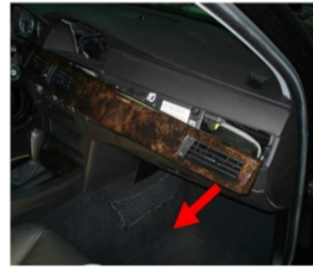
Open the cover with a tool.
