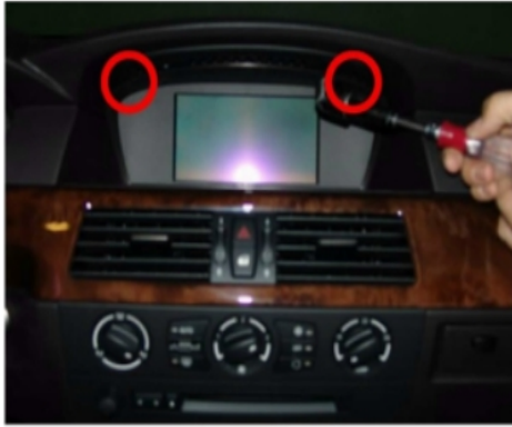
Loosen the screws of the monitor as indicated, remove the monitor, and unplug the connector.
