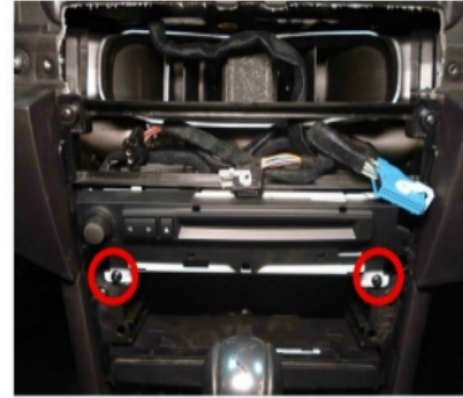
Loosen the screws of the MASK on both sides as indicated.
