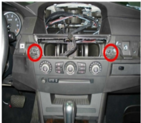
Loosen the screws on both sides as indicated.
