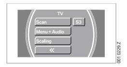
Use the automatic channel search if you are switching the DVB-T set-top box on for the first time or if the picture quality is poor on repeated occasions.
