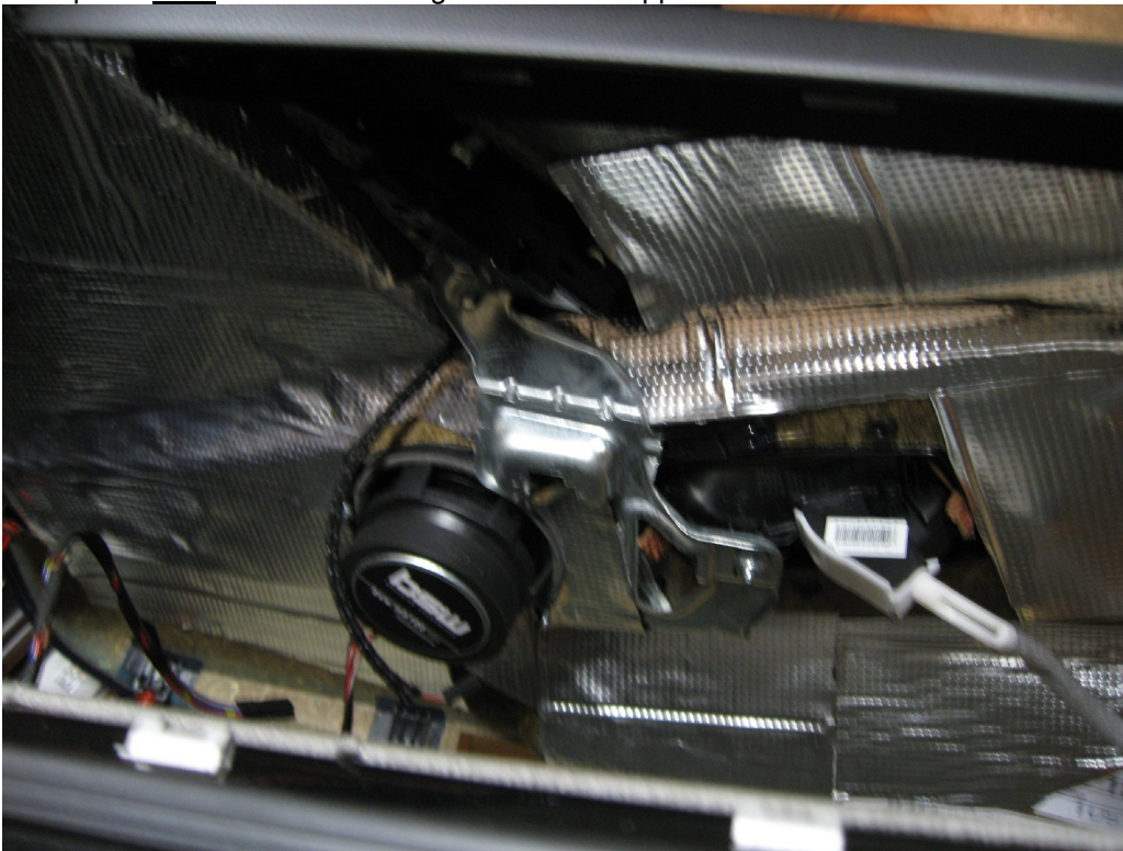
Door panel after sound deadening material was applied.
