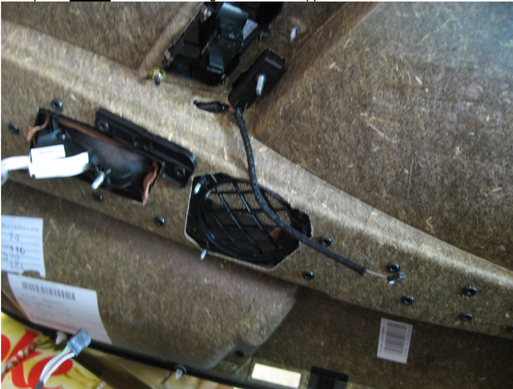
Door panel before sound-deadening material was applied.
