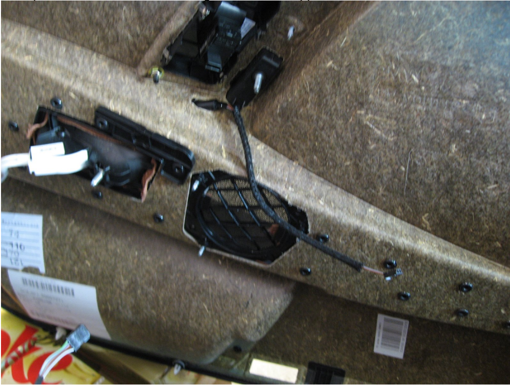
Door panel before sound deadening material was applied.
