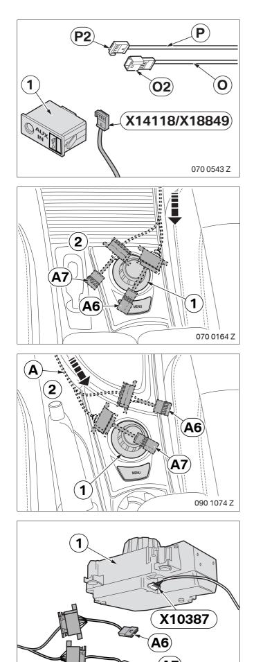
Route auxiliary cable **O** and **P** to the USB/AUX socket.
