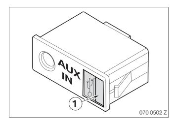
To play ACM audio through the car's speakers, please disconnect any devices that may be connected to the USB interface (1).
