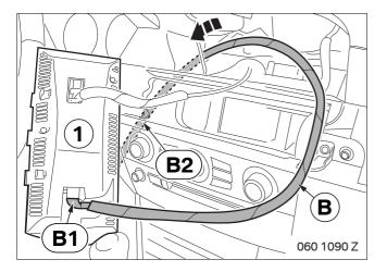
Connect branch **B1** (10-pin VI plug) of connection cable **B** on the control display (1).
