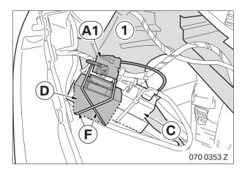
Attach Universal Can Interface **D** to the instrument panel (1) in front of the ACM unit **C** using cable ties **F**.
