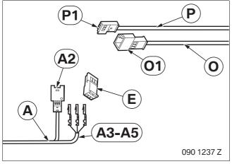
Route all branches except branch **A10** of the retrofit cable **A** along the standard wiring harness into the footwell on the front passenge side.
