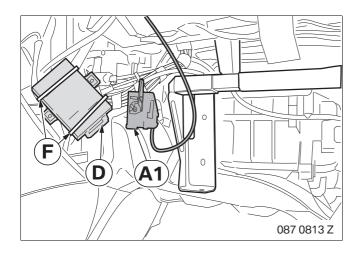
Secure Universal Can Interface **D** to the standard wiring harness using cable ties **F**.
