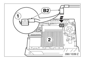
Remove coding (1) from branch **B2** (WS 10-pin plug). Connect branch **B2** (WS 10-pin plug) to the CCC (2) as shown.
