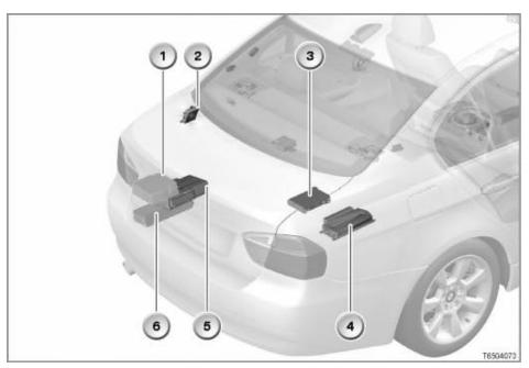
The illustration shows the installation location of the satellite tuner in the E90. The installation location is similar on the E91
