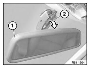
Twist mirror (1) at an angle towards front and left/top. Swivel right shell (2) off ball neck in direction of arrow; this detaches the engagement clip from the metal foot.
