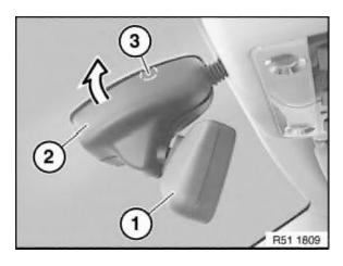
Twist mirror (1) at an angle towards front and right/top. Swivel left shell (2) off ball neck in direction of arrow; this detaches the engagement clip (3) from the metal foot.
