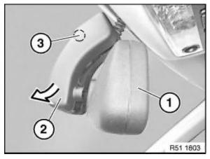
Twist mirror (1) at an angle towards front and right/top. Swivel left shell (2) off ball neck in direction of arrow; this detaches the engagement clip (3) from the metal foot.
