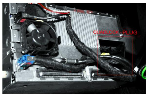
This QUADLOCK-plug is become accomplished with the multi plugs. From the big QUADLOCK-plug pulls out the white color terminal. The video transmission line fix.
