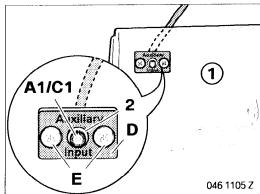
Insert branch **A1/C1** in the glove compartment (1) and secure it to the mounting plate **D** with a knurled nut (2).
