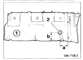
Drill a hole (2) in the trim (1) with a 3 mm twist drill bit through which you can thread the AUX connector wiring harness.
