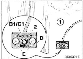
Insert branch **B1/C1** in the glove compartment (1) and secure it to the mounting plate **D** with a knurled nut (2).
