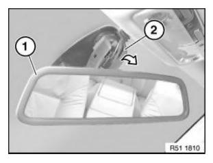
Twist mirror (1) at an angle towards front and left/top. Swivel right end cap (2) off ball neck in direction of arrow; this detaches the engagement clip from the metal foot.
