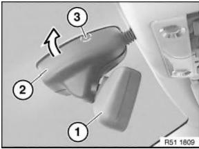
Twist mirror (1) at an angle towards front and right/top. Swivel left end cap (2) off ball neck in direction of arrow; this detaches the engagement clip (3) from the metal foot.
