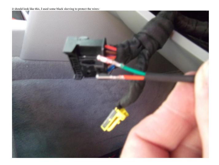
Plug it all back in and cable tie the wires. Lastly you need to run the wire from pin 12 (green) to ground, I used the grounding point underneath the bonnet release lever under the carpet using a 6mm lug:
