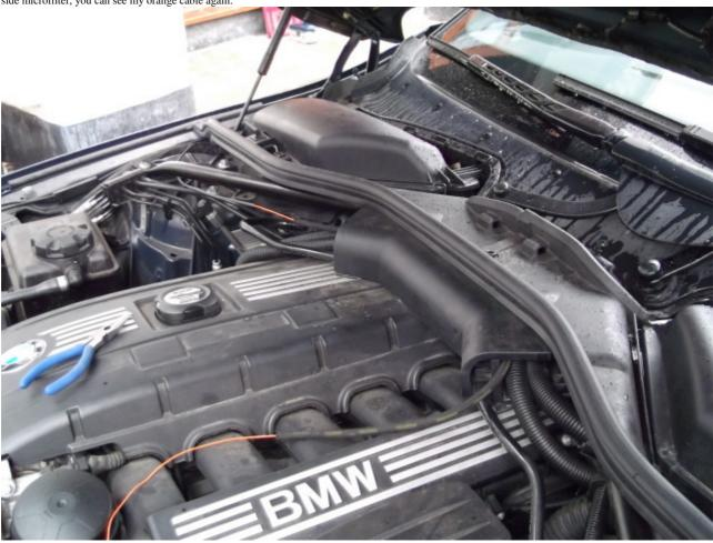
This is the ebox underneath the passenger microfilter where the cable needs to end up, you can see I routed the cable through the rubber flexi hose, you can see that I simply located the correct wire and put a crimp lug on to join it:
