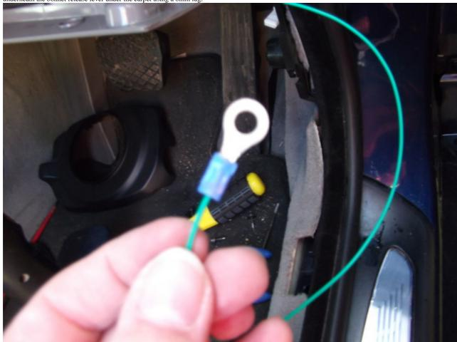
You can just see the black plastic cover over the earth point under the carpet, there is a 6mm bolt to put the lug onto:
