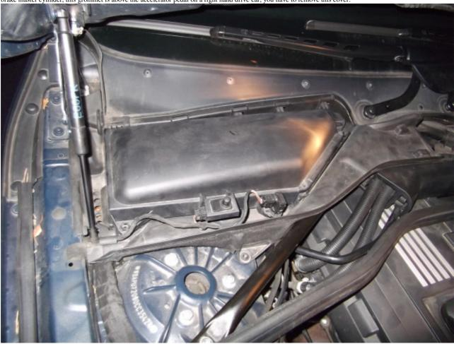
This is whats underneath, you can see my new orange cable which I just pushed through the rubber grommet and left it long inside the underdash trim at this stage:
