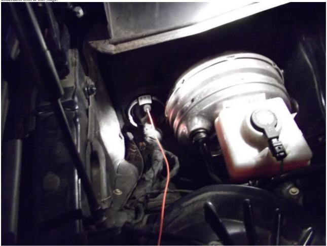
I routed this cable along the strut brace inside a piece of vacuum hose to protect it, the cable needs to go to the e box under the passenger side microfilter, you can see my orange cable again:
