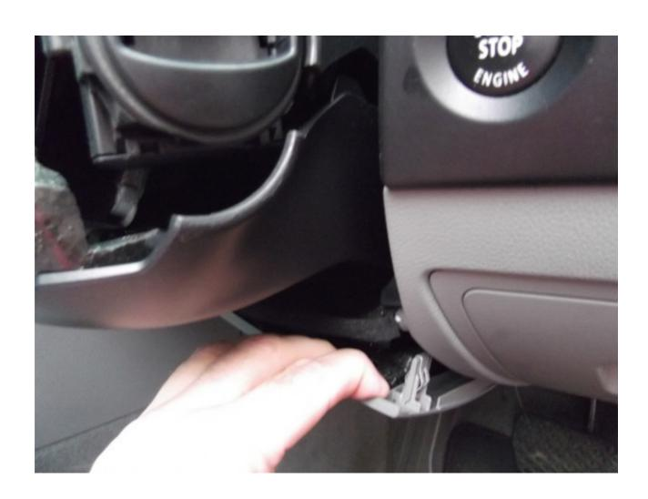
Next locate the SZL connector X1880 under the steering column next to the yellow connector (this shows the connector with the new wires in place):
